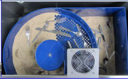
The cutlery is spirally transported upwards through a high-grade granular substance and is dried and polished. The installed ventilator prevents that granulate comes out of the machine.
